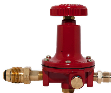
PART No. 1230VK2 0-30 PSI ADJUSTABLE INLET POLXF OUTLET MALE 3/8" SAE CAPACITY 900,000 BTU
