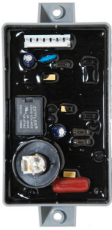
S-415P - IGNITION BOARD S-415W - WIRING HARNESS (F-400T, F-1000T, F-1500T)
