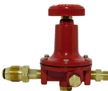
PART No. 1230VK1 0-30 PSI ADJUSTABLE INLET POLXF OUTLET MALE 9/16"-18LH CAPACITY 900,000 BTU
